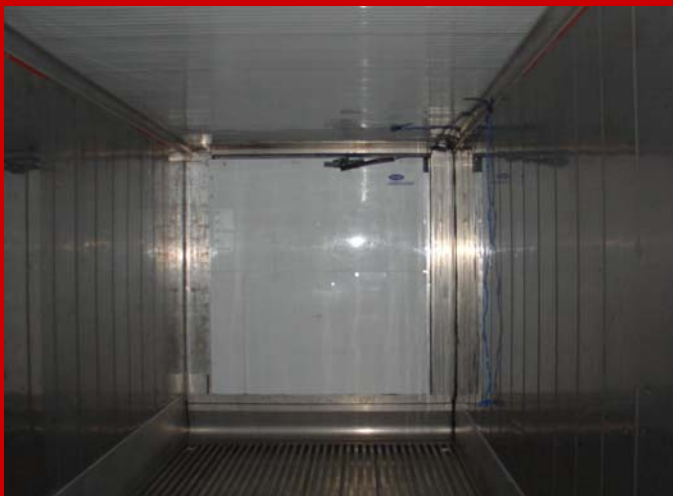
Typical internal view showing Airflow floor and front bulkhead with bottom air delivery and top air return panels. Also shows position of maximum cargo height line when container is used for refrigerated or temp controlled cargo (usually 100 mm from top in 6M container and 150/200mm for 12M container).
